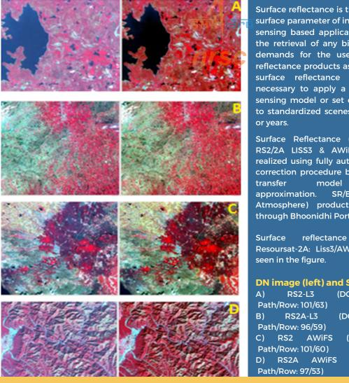
Surface reflectance is the fundamental land surface parameter of interest for any remote sensing based application. This is because the retrieval of any biophysical parameter demands for the use of precise surface reflectance products as the input. Moreover surface reflectance products are also necessary to apply a quantitative remote sensing model or set of classification rules to standardized scenes in different regions
